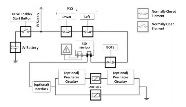
The shutdown circuit directly carries the current driving AIRs. If the shutdown circuit
